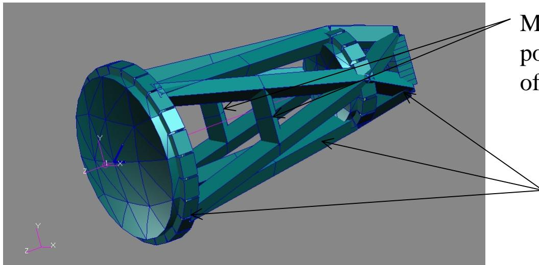
Displacements of the three optical elements are shown in blue.
