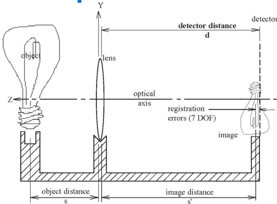
**Ivory** determines changes in the position, orientation and size of the image on the detector.
