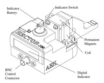
be subdivided into very small fractions of the calibrated range, providing physical displacements from about 200 nanometers sizes to under 1/10 nanometer sizes as desired. HECTOR-100 may itself be calibrated in an optical interferometer which makes its artifacts traceable to the SI unit of length (the wave length of light). The artifacts may be accurate and repeatable to 1 part in 1,000 or better, depending upon the procedures employed.
